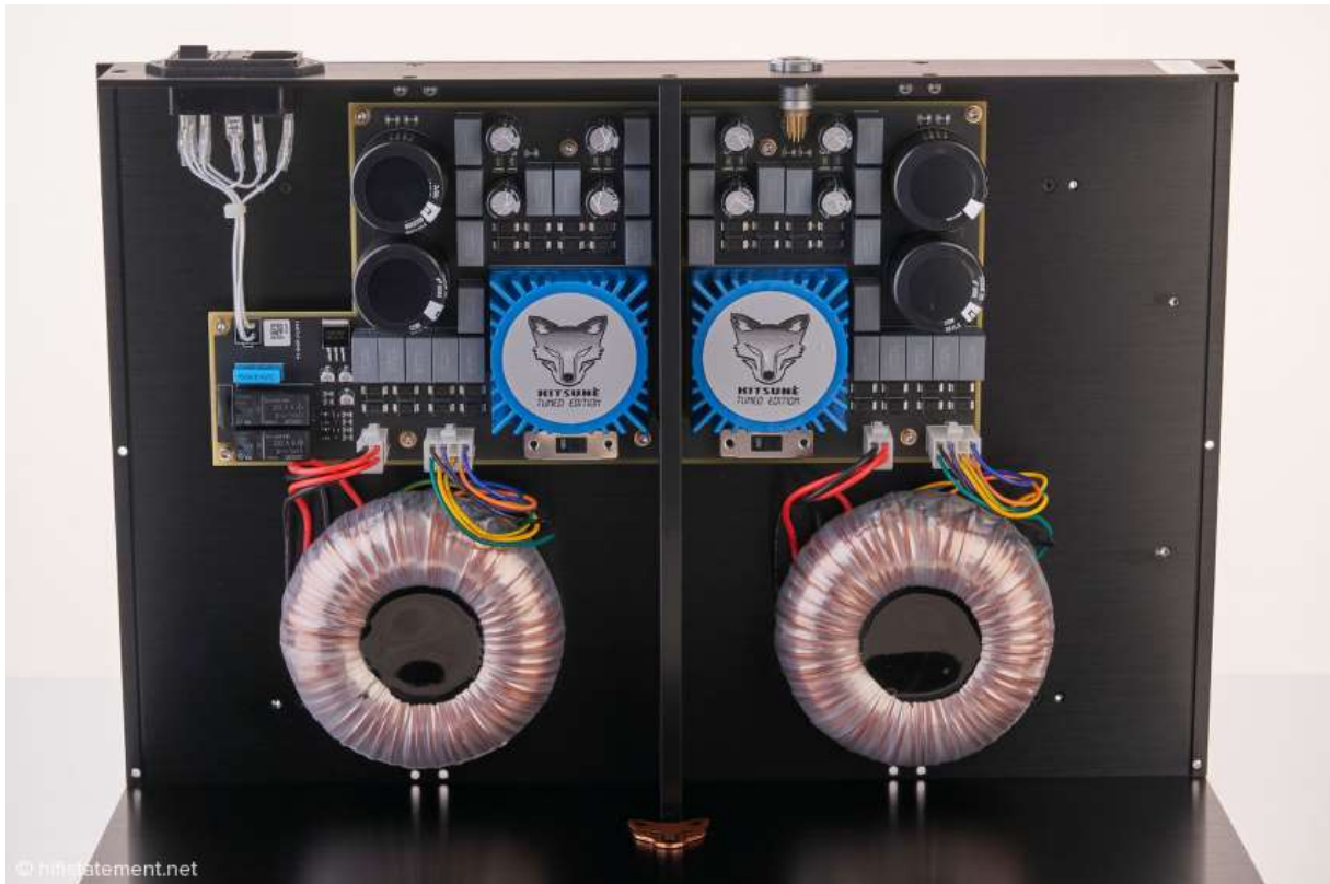
The separate power supply for each channel
